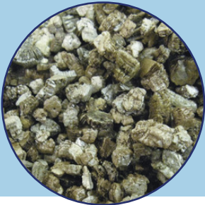
VERMICULITE / BLOWN INSULATION
